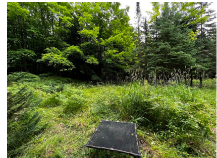
This seed trap sits in an open area at one of Kiley's sites. She used these to capture seeds falling from the trees she studies, which are mostly white spruce, balsam fir, sugar maple, and white pine. These traps allow seed production and dispersal to be quantified.
